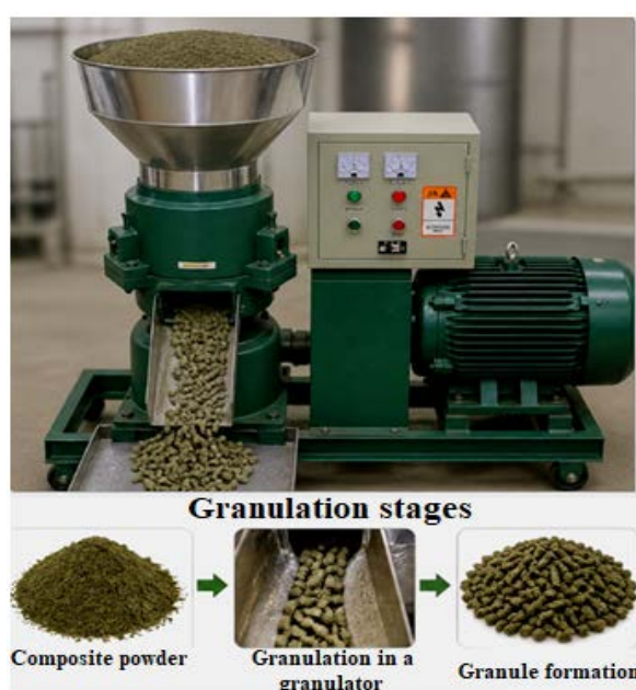
Fig. 2. Granulation stage of the organo-mineral biocomplex
